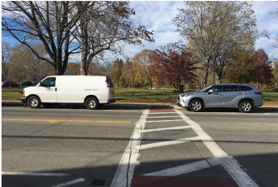
Figure 15: Parking too close to the crosswalks resumed once the delineators were removed
